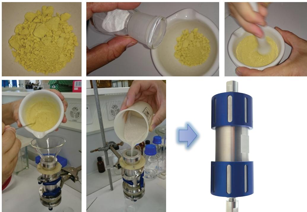
1. Adsorb the dissolved sample in a "better solvent" on a small amount of stationary phase (Silica, C18 or Celite).
