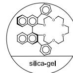
These columns contain a chiral crown ether as a chiral selector, which is coated onto a 5  $\mu\text{m}$  support. Acidic mobile phases such as Perchloric acid pH 1 to 2, are used to operate these columns under standard conditions. Note that to shorten the retention time of hydrophobic samples, the addition of Methanol (15% maximum v/v) has been shown to be effective.
