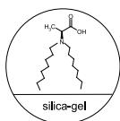
The Chiral Stationary Phases in these columns are made of amino acids and its derivatives coated bonded to silica supports (with a particle size of 10  $\mu\text{m}$  for WH and 3  $\mu\text{m}$  for MA(+)). Since these columns are ligand-exchange type columns, the standard mobile phase to use is an aqueous solution of CuSO<sub>4</sub> (0.1 to 2mM). These columns can tolerate organic modifiers such as Methanol and Acetonitrile according specifications in the instruction manual.
