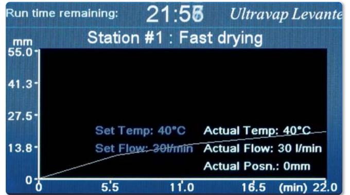
▲ The informative run-time display shows the progress of each evaporation run with real-time information on gas temperature, gas flow rate, stage position and remaining run-time, with an easy to read cursor display.
