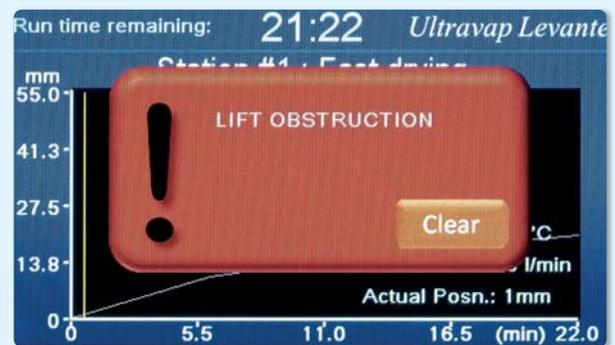
▲ Audible and visual warning of any obstruction is clearly shown and must be cleared by the user or the remote operating system for maximum safety.
